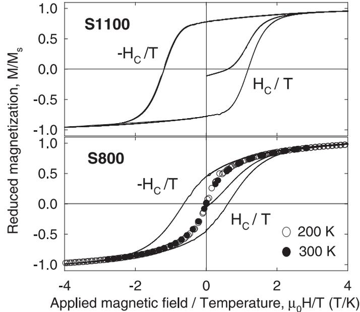
**Figure 3.** Virgin magnetization curves and hysteresis loops of S800 and S1100 samples measured at 2 K (solid line) together with unhysteretic curves of S800 in SPM state. The deviation of the virgin curves from the expected zero value at 0 T is due to a small fraction of the sample being already magnetized.
