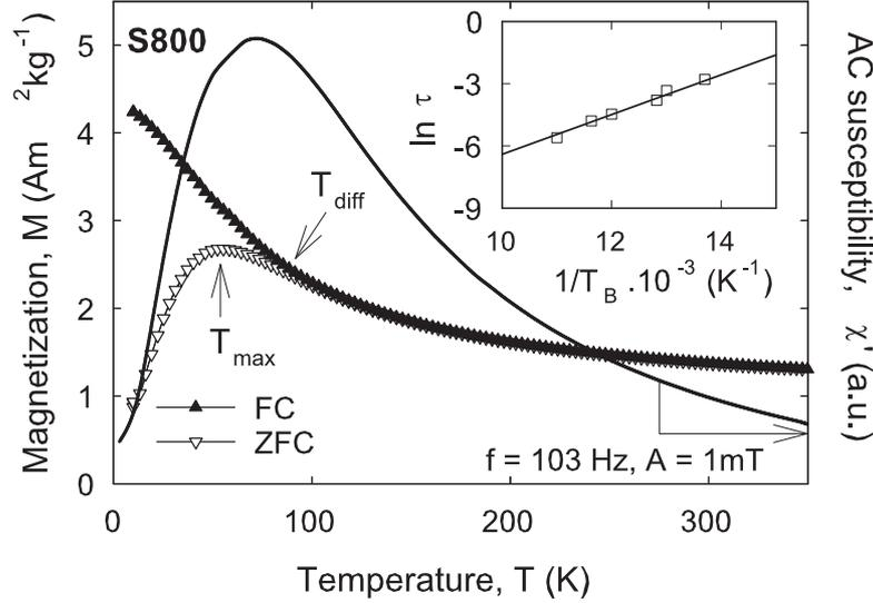
**Figure 2.** Temperature dependence of ZFC - FC magnetization of S800 sample at 50 mT in comparison with that of AC susceptibility (real part,  $\chi'$ ). The inset shows the logarithmic dependence of the relaxation time  $\tau$  against the inverse blocking temperature  $T_B$  according to the Néel - Arrhenius law.
