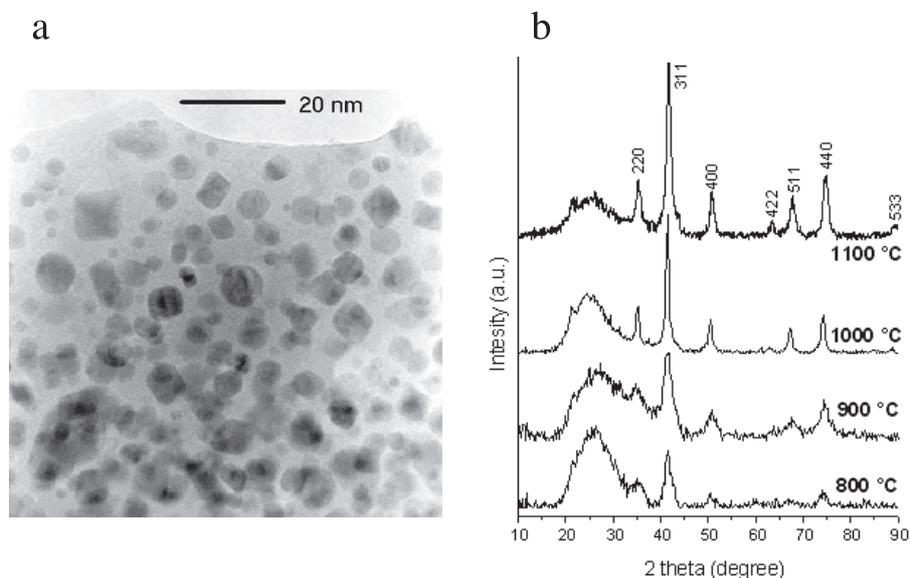
**Figure 1.** a - HR TEM image of S1000 sample. b - XRD patterns of S800 - S1100 samples. The extended maximum at  $\sim 25^\circ$  corresponds to the amorphous silica matrix contribution.
