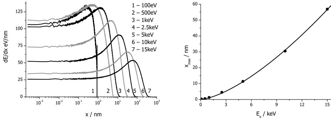
**Figure 6.** A modelled amount of a lost beam energy as a function of depth in a planar sample (left) and its maxima position as a function of a beam energy (right). As for the noise, see the note in Fig. 5. The fit equation is  $x_{max} = 1.0 E_e^{3/2}$  (in plot units).
