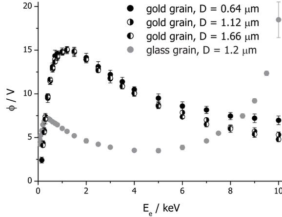
**Figure 8.** Experimental equilibrium characteristics of the secondary electron emission for a spherical glass grain and spherical gold grains of different diameters. The position of the first maximum is driven by surface emission properties. On the other hand, the increase of a potential at high beam energies is dominantly determined by a grain size – it needs to be comparable to a beam penetration depth.
