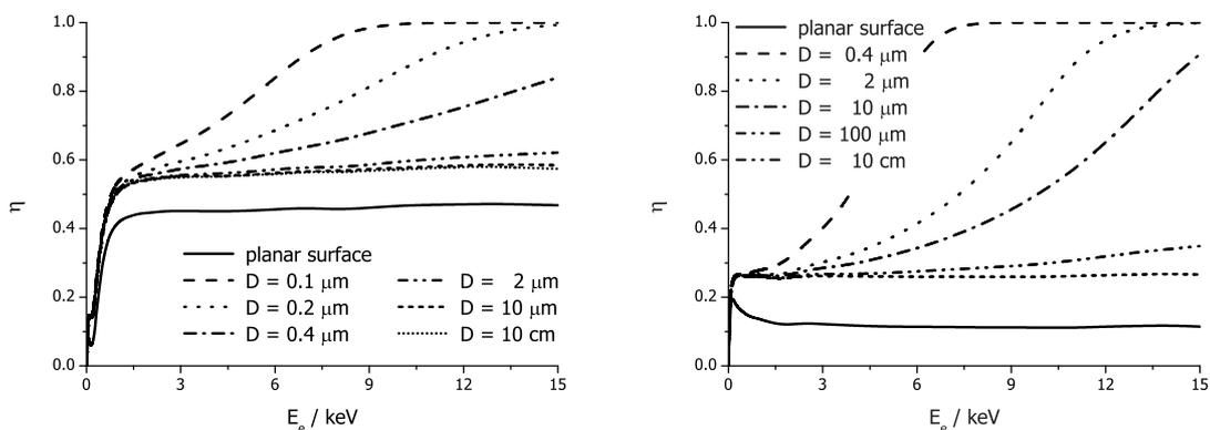
**Figure 9.** A modelled BE yield for samples of different sizes for glass (left) and gold (right). Whereas  $\eta$  enhancement at higher energies occurs for gold grains only at diameters smaller than  $\approx 2 \mu\text{m}$  in a given energy range, it is appreciable until  $\approx 100 \mu\text{m}$  diameters for glass grains.
