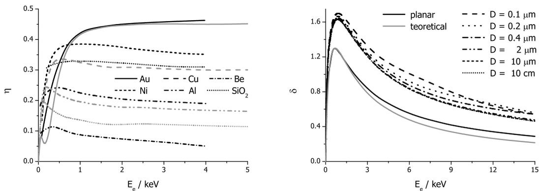
**Figure 7.** Left: An example of experimental [Bronstein and Fraiman, 1969] (black) and modelled (grey) BE yield curves for several bulk materials at a normal incident angle.  $\eta$  almost does not change above a few keV. Right: A modelled SE yield for gold planar sample and grains of different diameters.  $\delta$  depends on a diameter for grains smaller than  $\approx 0.5 \mu\text{m}$  only. The Draine and Salpeter [1979] universal curve is used.
