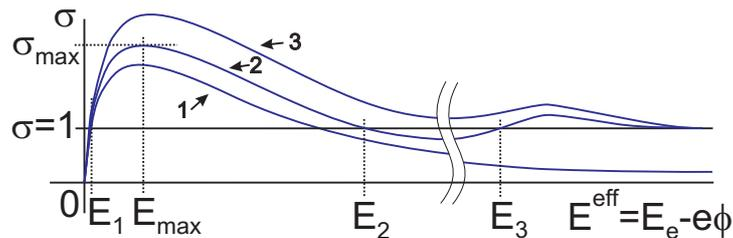
**Figure 1.** Schematics of the total secondary yield dependence on an effective beam energy: (1) a large planar surface, (2) a dust grain from the same material, and (3) another dust grain with a higher value of the SE yield maximum. The SE yield enhancement leads to positive equilibrium potentials for high energies. Note that for very high energies  $\sigma$  approaches  $\eta$  which is equal unity for dust grains as no PE can be calmed down in such a tiny piece of matter.
