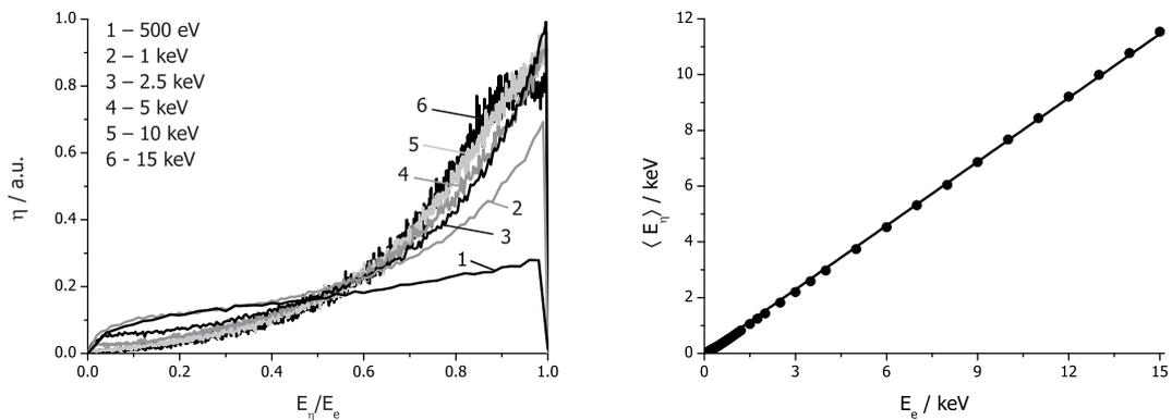
**Figure 5.** Left: Relative modelled spectra of scattered electrons for a planar sample. Note that the noise results from a statistic error which decreases with a number of PEs,  $N$ , as  $1/\sqrt{N}$  ( $N = 10^7$  used here). Right: A mean energy of scattered electrons (obtained from data similar to that presented in the left figure) as a function of a beam energy. The linear fit slope was determined to be 0.76.
