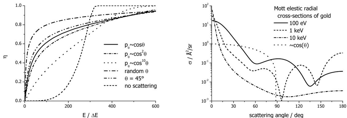
**Figure 2.** A BE yield as a function of an energy for different deflection distributions at a collision ( $\Delta E \approx 35$  eV) (left) and comparison of Mott elastic radial scattering cross-sections of gold [*Mott and Massey, 1965; Czyżewski et al., 1990*] to the cosine distribution (right). The main difference between models is an angular cross-section dependence.
