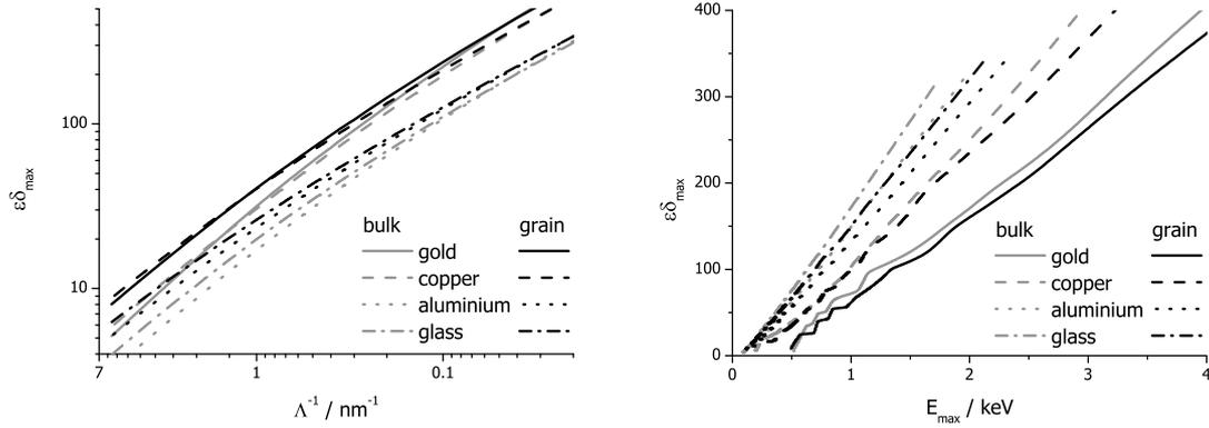
**Figure 4.** A modelled dependence of a SE yield maximum on the mean free diffusion path of secondaries (left) and on the energy corresponding to the maximum (right) for several materials. Planar samples and 10 cm grains are used. Note that  $\delta_{\max}$  is plotted in  $\varepsilon$  units. Some curves are coarse due to an error caused by a procedure of establishing of the maxima.
