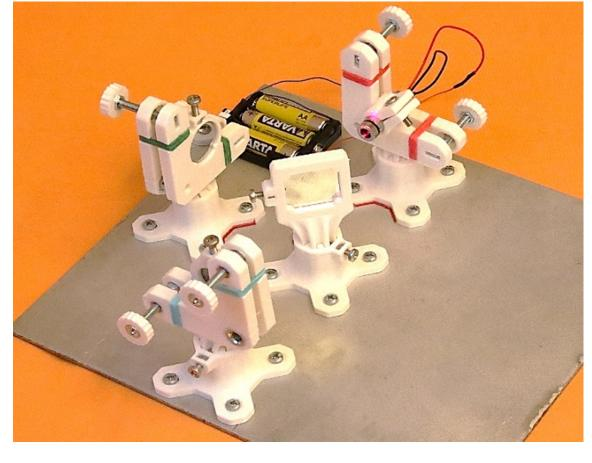
Furthermore, a functioning model of a Michelson interferometer, created by means of 3D-printing will be exhibited, while the building instructions have already been made public on the Internet. Additionally, several experiments with UV and IR radiation, luminescence of liquids and formation of Lichtenberger patterns will also be presented.
