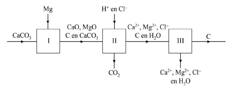
Schools lack Argon-ovens. However, the principles of graphene production can be shown quite easily using an excess of Magnesium. Here we present a chemistry experiment that can be used in school settings.
