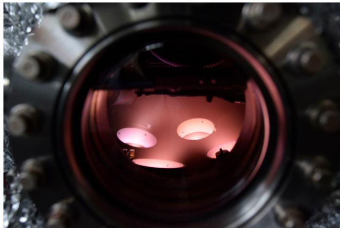
Figure 1: Magnetron sputtering system with ignited plasma for thin film deposition
