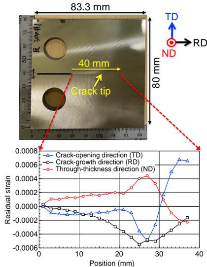
Fig.1 Residual strain determined via neutron diffraction.
