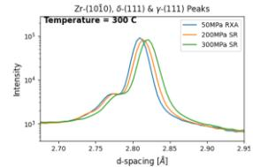
Figure 3: Presence of the  $g$ -(111) peak under load and temperature
