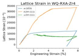
Figure 1: Extreme strain in  $d$ -(111) and appearance of  $g$ -(111)
