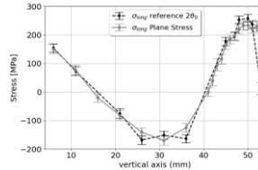
Figure 2: comparison between the longitudinal stress calculated under plane stress and with reference  $2\theta_0$  at the section V55.
