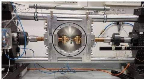
with EPICS through MQTT. The rig will allow performing deformation tests with a strain rate in the range of  $10^{-3}$ -100 mm/min. Various types of holding grips will be developed with respect to the shape and the size of testing samples.
