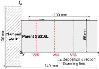
Figure 1: location of the lines (red) where were performed the neutron strain measurements.
