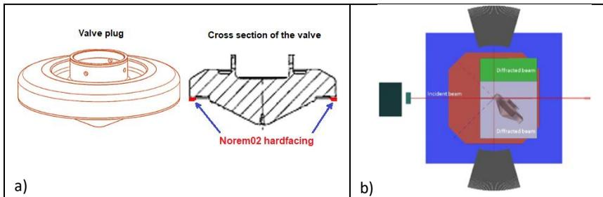
Figure 1: a) Nuclear plant Valve plug with Norem02 hardfacing, b) Simulation of Neutron diffraction residual stress measurements.
