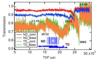
Fig.1 Bragg-edge spectra obtained from TD and ND for the base plate and FSSW joint region.
