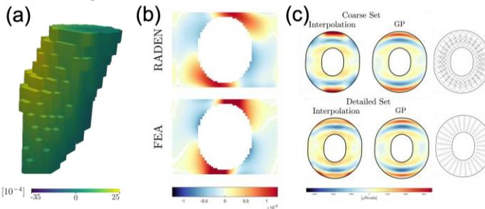
Figure 4: (a) Reconstructed  $e_{\{xx\}}$  intragranular strain for a columnar tin grain from scanning-3DXRD [2]. (b) Triaxial strain reconstruction from neutron transmission measurements [1]. (c) Strain estimation of a plane stress crushed ring from neutron diffraction measurements [3].
