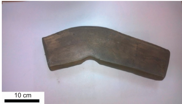
Fig. 4.5.13 Ti-6Al-4V prepared by ECAP. Semi-product for hip implant manufacturing.
