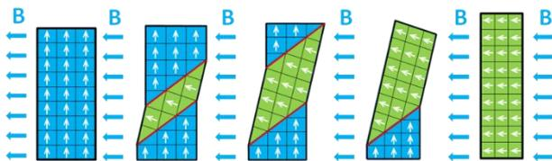
*Figure 1. Illustration of the reversible nature of sizeable strain in single crystalline Ni-Mn-Ga, by twin boundary motion. **Upper**, the MIR effect by application of magnetic field, **lower**, recovery to the original shape by applied force.*
